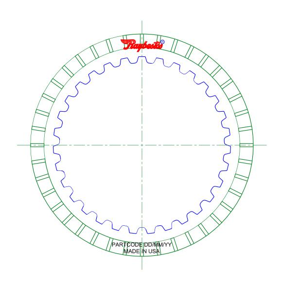
FRICTION PLATE SPECIFICS **APPLICATION** NUMBER OF TEETH Year Coverage 31 **Transmission** Clutch Pack **OUTSIDE DIAMETER** 4.770±.010 **62TE** 2007 - UP **UNDERDRIVE LOW** FRICTION MATERIAL HI ENERGY GREEN **OVERALL THICKNESS** .073 (OE REF) DRAWING SCALE PART NUMBER
