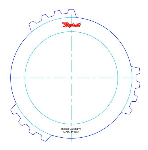
FRICTION PLATE SPECIFICS **APPLICATION** NUMBER OF TEETH Year Coverage 12/30 **Transmission** Clutch Pack **OUTSIDE DIAMETER** 4.399±0.005 4T65E 3rd 2001-UP FRICTION MATERIAL **GREEN** OVERALL THICKNESS 0.078±0.003 DRAWING SCALE 1:1
