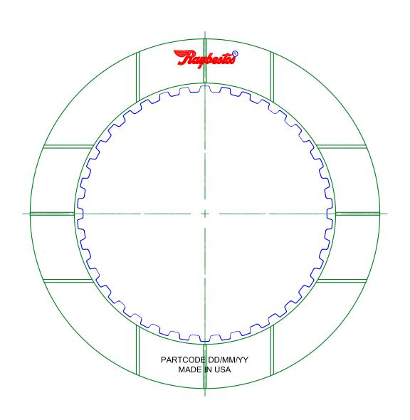
FRICTION PLATE SPECIFICS **APPLICATION** NUMBER OF TEETH Year Coverage 38 **Transmission** Clutch Pack **OUTSIDE DIAMETER** 5.118±.010 4T60E **SECOND** 1994**-**UP FRICTION MATERIAL **GREEN** OVERALL THICKNESS .069±.003 DRAWING SCALE 1:1
