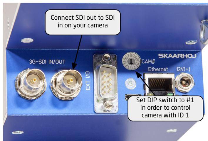
Notice, using the SDI output means the RCP does not know what settings the camera already has. So any parameter set for the first time may result in a “jump” in settings on the camera. After that they should be absolutely smoothly adjusted.
