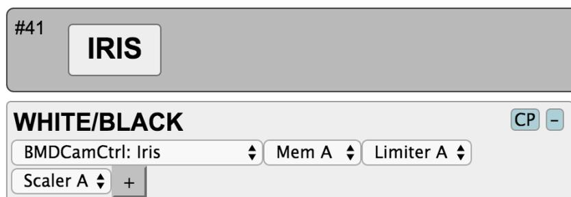
It's very easy to change your RCP to select camera in a different way. Lets assume you want the 6 user defined buttons U1-U6 to select camera instead. First you disable the Cam Select components function by selecting a blank function in the top:
