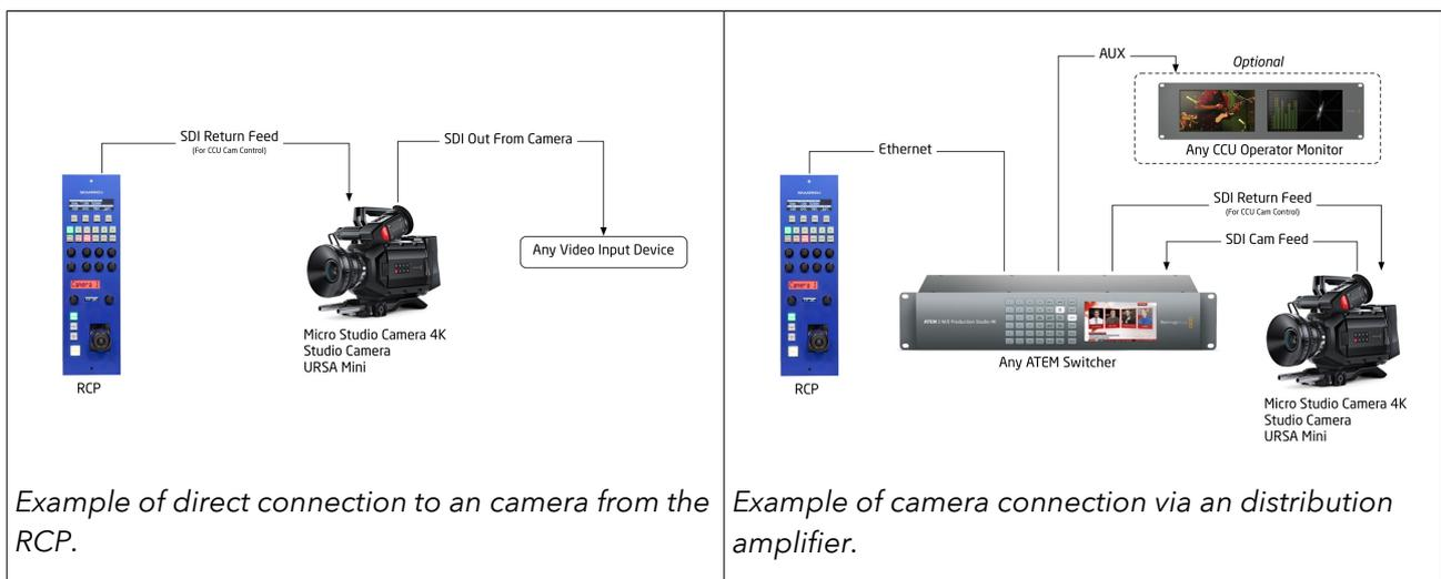
In any case, the RCP must be set to the same camera ID as the camera it's supposed to control.
