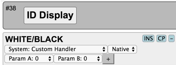
If you change this configuration accordingly, the name and tally status of input X on the ATEM switcher will be shown instead (where X is the camera number stored in Mem A - you could also set it to a different input number if you please):
