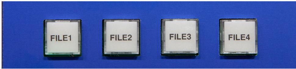
Press any of these and if CCU settings are stored in this particular memory bank, it will be sent to the camera. At this point the button will blink for 10 seconds and if you push the button again within this period of time you will revert back to the settings you had before you pushed the button.
