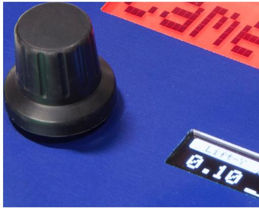
On the right you will find the limiter. This knob limits the range of the iris control knob or handle. The right side of the OLED display shows the current iris value in percent. The bar below the number has tiny indicators that show where the limits are if you apply them. The limits basically sets a limit to how far you can adjust the iris value in both the high and low ends. You toggle between changing the high and low ends by pressing the knob down.
