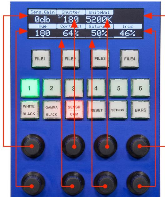
As you press the three keys “White/Black”, “Gamma/Black” and “Sensor/Cam” you will see the content of the tiles change. This is the three “menu states” of the controller.
