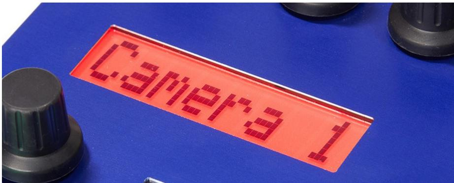
This will show you the camera number selected on the Cam# selector under the bottom. If pin 8 on the DB9 plug is shorted to ground (pin 5 or 9), it will change color to red instead of white.
