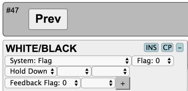
This configuration means that for as long as the button is pushed, Flag 0 in the controllers internal memory is set true (and the button will light up for as long as Flag 0 is true).
