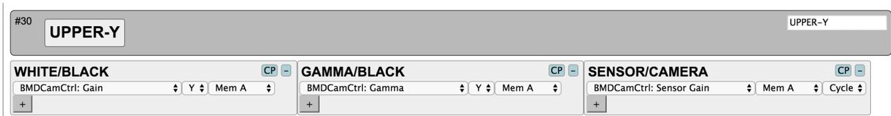
In case the first menu state activated by the "WHITE/BLACK" button, the knob will adjust luminance gain (high lights = white), otherwise if "GAMMA/BLACK" is activated it will adjust luminance Gamma (midtones) and in the third case of "Sensor/Camera", the sensor gain (db) is adjusted.
