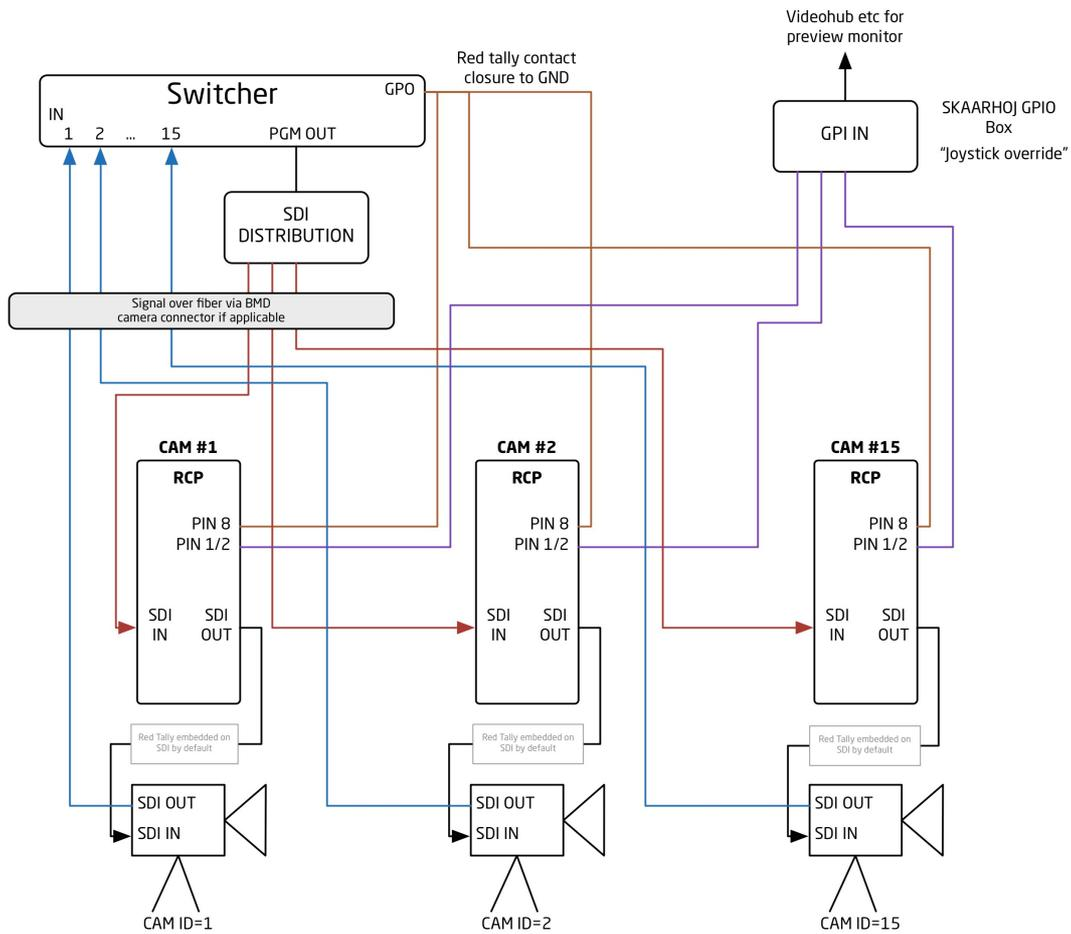
Even though the RCP will work without an SDI input, it's recommended to feed one. Only for cameras like the Micro Studio Camera where you have no viewfinder on the camera it makes no sense, but otherwise the SDI input is forwarded on the SDI output to the camera so the camera operator can see the return feed picture on his viewfinder.
