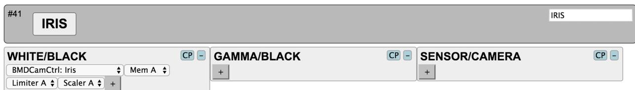
As you can see, there are no function in the "Gamma/Black" and "Sensor/Camera" columns but since the principle is to fall back to the first columns action, the iris joystick therefore does not change its function as you change the controller state.
