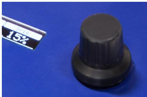
The Iris joystick is the iconic hardware interface component known from professional CCUs for all major camera brands. It has a back/forth slider function as well as a ring on the bell. If you push and pull the joystick you will adjust iris while if you turn the ring you will adjust the master black level. On top of the joystick you will find a button and if you push it, you will toggle the relay on the DB-9 connector ("Joystick override").
