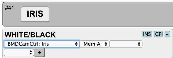
It instructs the iris joystick to send iris control commands over SDI out (Blackmagic Camera Control protocol) for the camera with the ID currently stored as a value in "Mem A" in the RCP (see section on camera selection).
