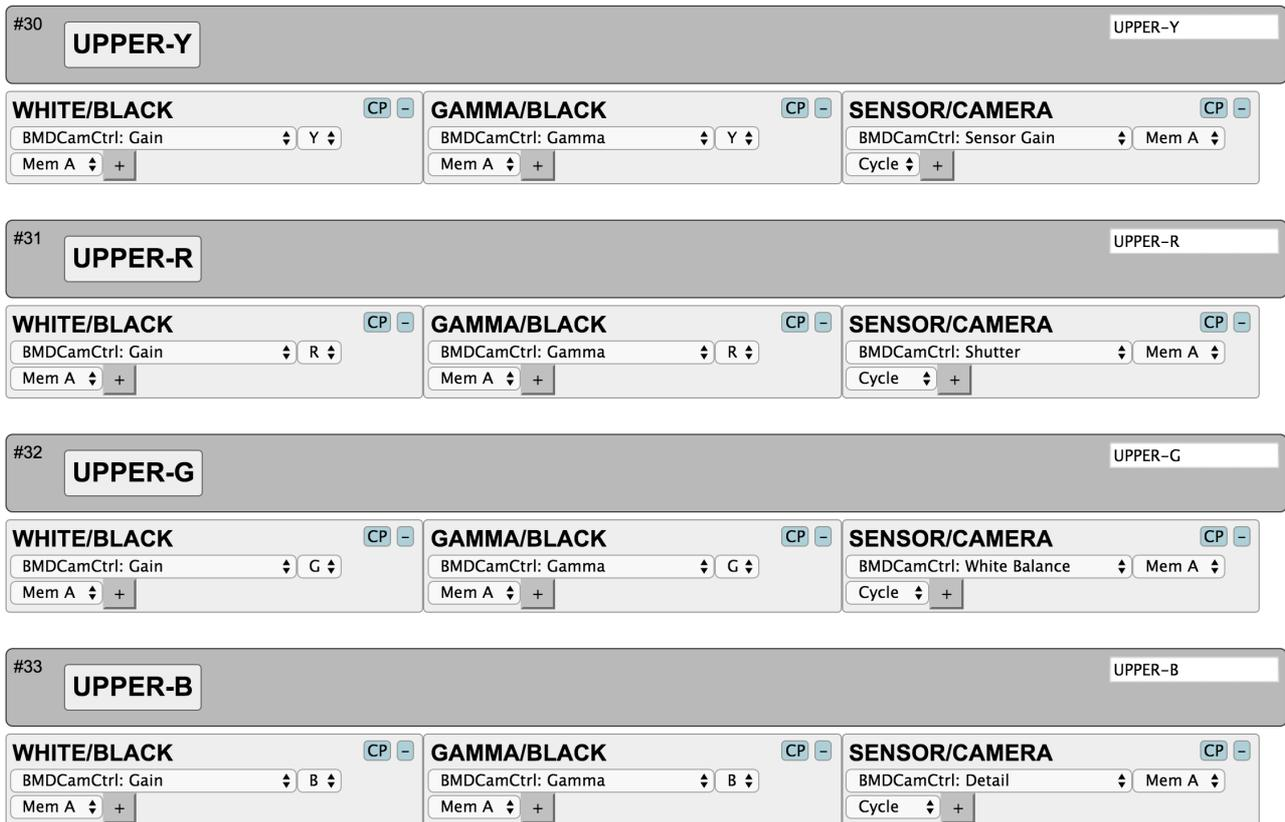
Changing how the various parameters are organized in the menu is now a simple matter of adding and removing actions within this framework. You can even add a fourth menu button setting up state "3" by adding a new state in the "States" section. This will result in yet a column of actions.
