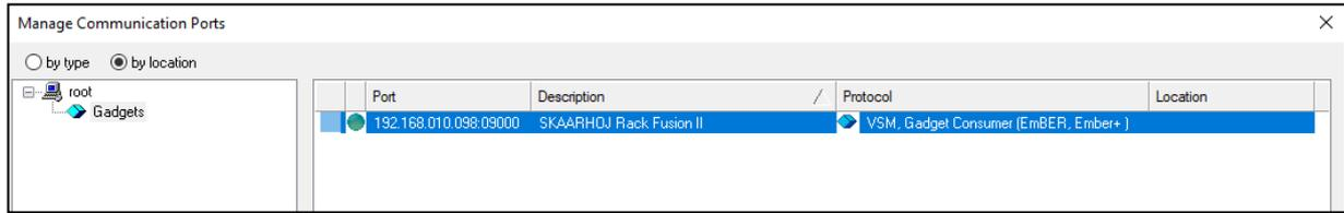
If no project is open, the connection indicator will often light yellow. Any interaction with the SKAARHOJ controller (such as pressing a button, will typically turn the connection status to green)
