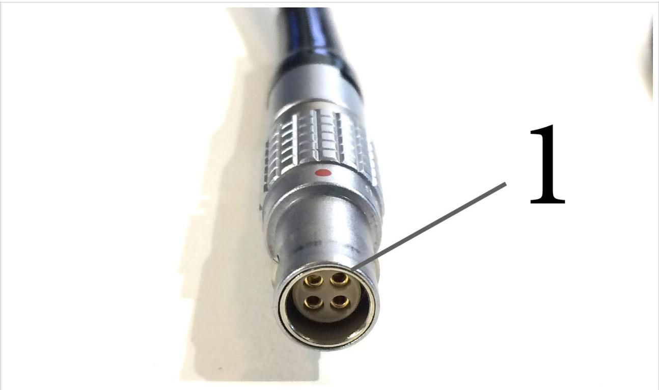
Looking into the female connector on the wire to the Flare camera with red dot on 12 o'clock, pin 1 (as we define it here) is at 1:30 o'clock and then clockwise:
