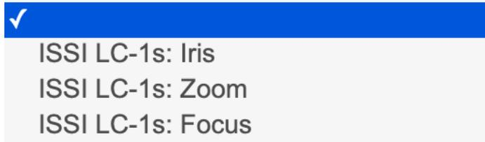
For each of the 3 actions there is a “balance/speed” value that can be set as well. This can either be set to a fixed value or the balance/speed value can be set to a Memory parameter (K-N) which then can be controlled elsewhere on a controller to have on the fly adjustments. Find a value suited for your lens.
