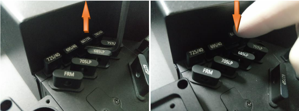
Figure 29. Change the Optical Filter
