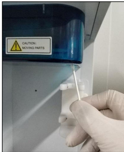
Figure 86. Wipe the SIP Cleaning Apparatus' Lower Surface
