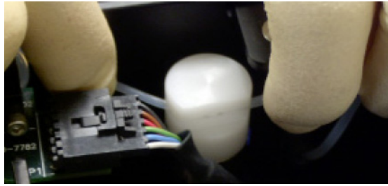
Figure 9.29 Tubing in Pinch Valve Slot
