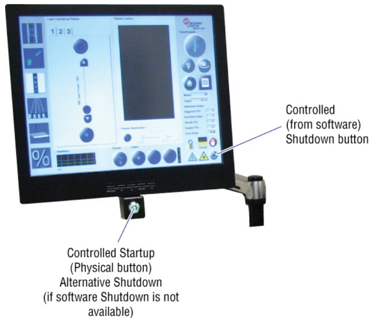
Figure 3.1 aXcess Control Panel Startup and Shutdown Buttons
