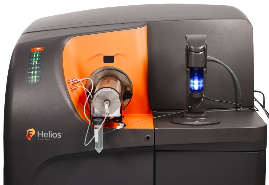
Figure 25. Sample Loader and sample heater assembly
