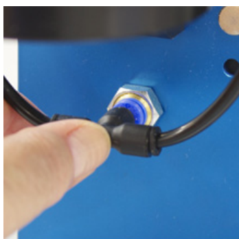
figure 1-44. Reconnecting the pneumatic supply
