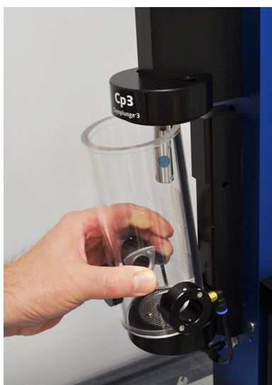
figure 1-43. Replacing the humidity chamber
