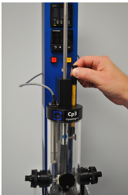
figure 1-14. Inserting the humidity wand
