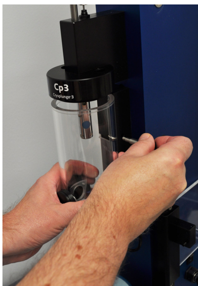
figure 1-42. Removing the humidity chamber
