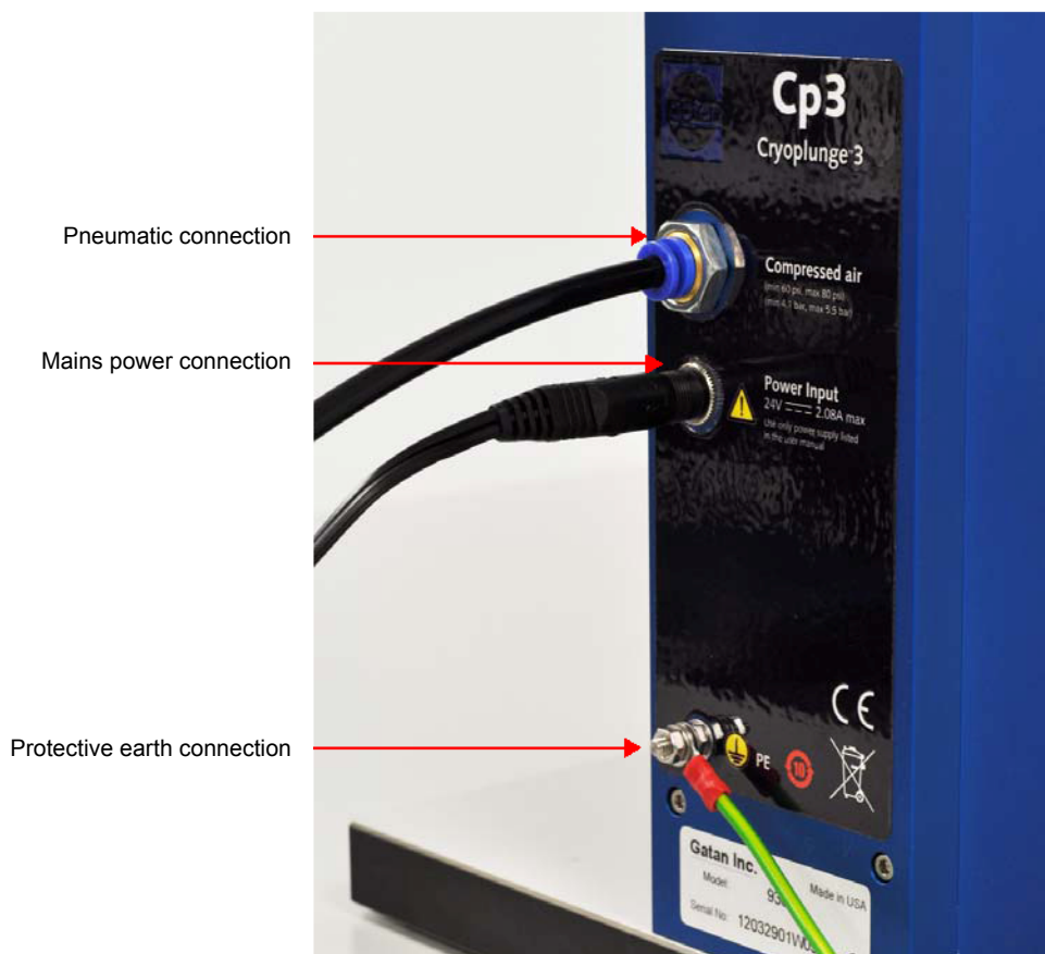
figure 1-9. Pneumatic, mains, and protective earth connections
