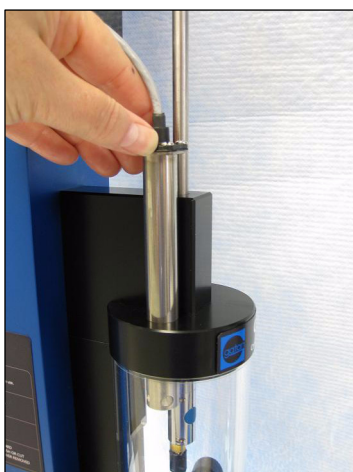
figure 1-12. Insertion of Omega temperature/humidity sensor
