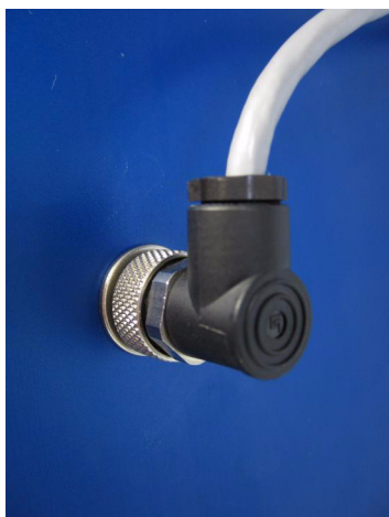
figure 1-13. Omega temperature/humidity sensor connector
