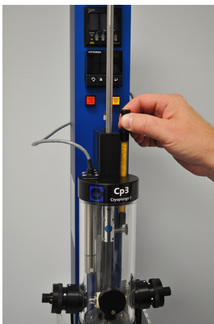
figure 1-39. Removing the humidity wand
