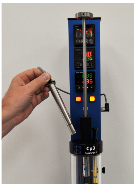
figure 1-40. Removing the temperature/humidity sensor
