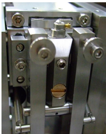
Figure 17. The outer allen washer screws on the knife arm.
