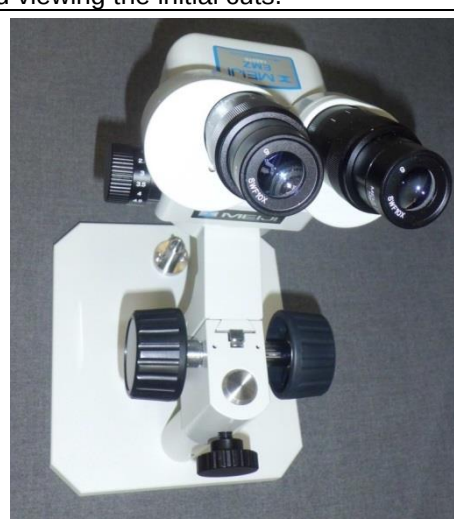
Figure 30. Optical Zoom Stereo Microscope attached to bench top mount.
