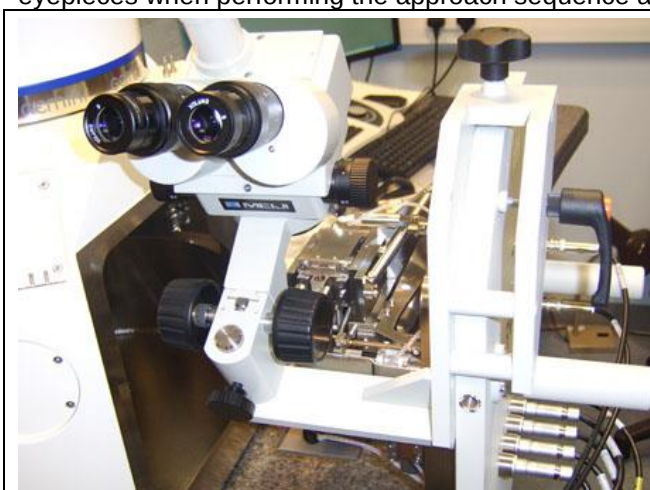
Figure 29. Optical Zoom Stereo Microscope mounted on SEM door.
