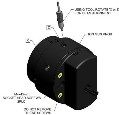
Figure 3-41 X and Z-alignment device screws
