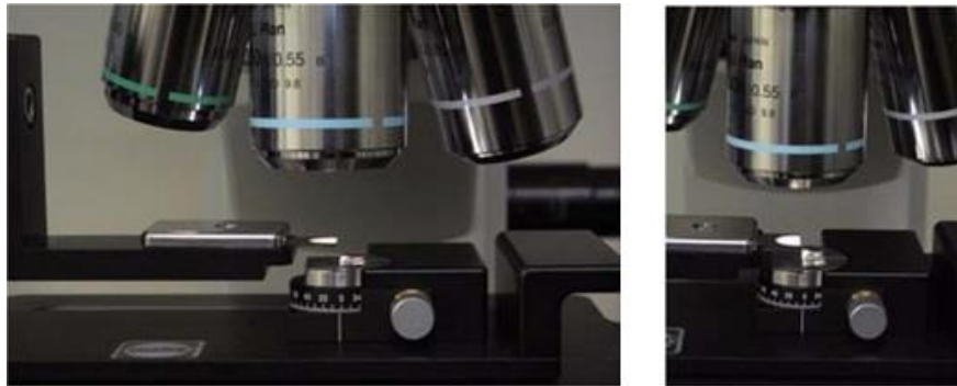
Figure 4-42 Site-specific loading dock on Light Microscope stage
