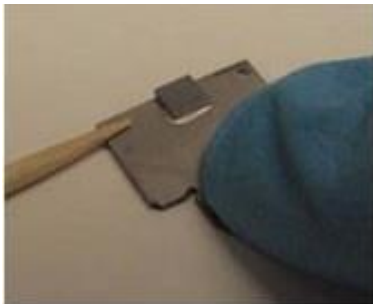
Figure 4-14 Scoring the Ag paint for specimen removal
