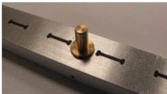
Figure 4-9 Bottom of Multi-sample blade SEM stub with pin stub
