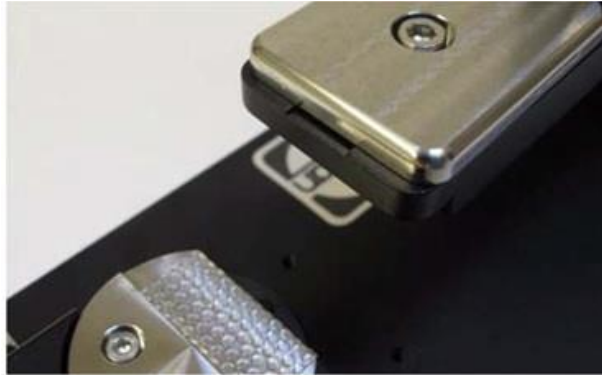
Figure 4-39 Blade mount clamp
