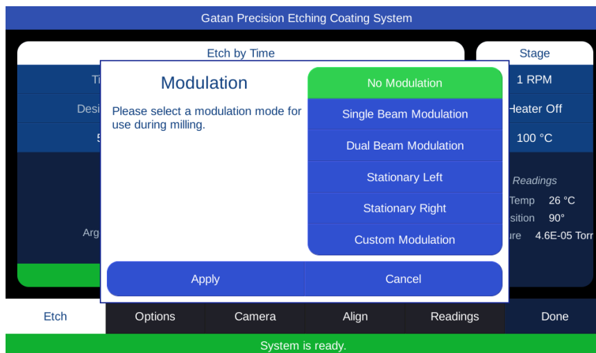
Figure 3-7. Setting Beam Modulation.
