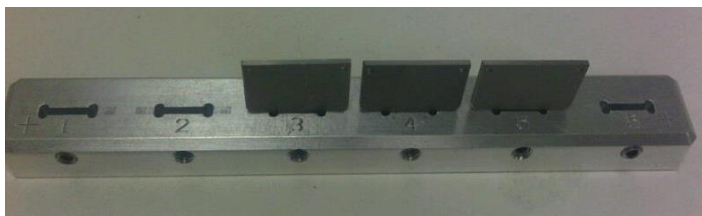
Figure 4-8 Multi-sample Blade SEM stub
