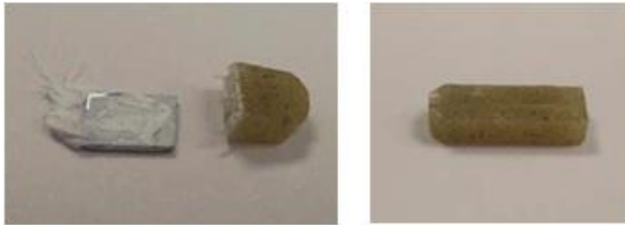
Figure 4-19 Casts removed from the Silicone Mold
