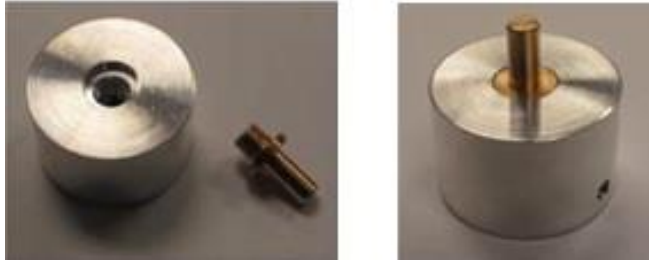
Figure 4-12 Pin Stub of single sample SEM stub
