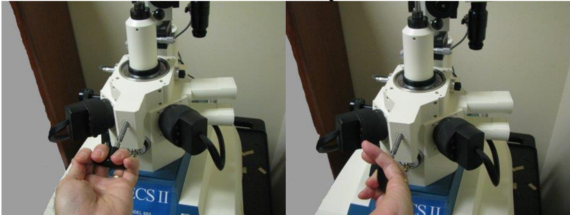
Figure 3-59. Opening the gate valve
