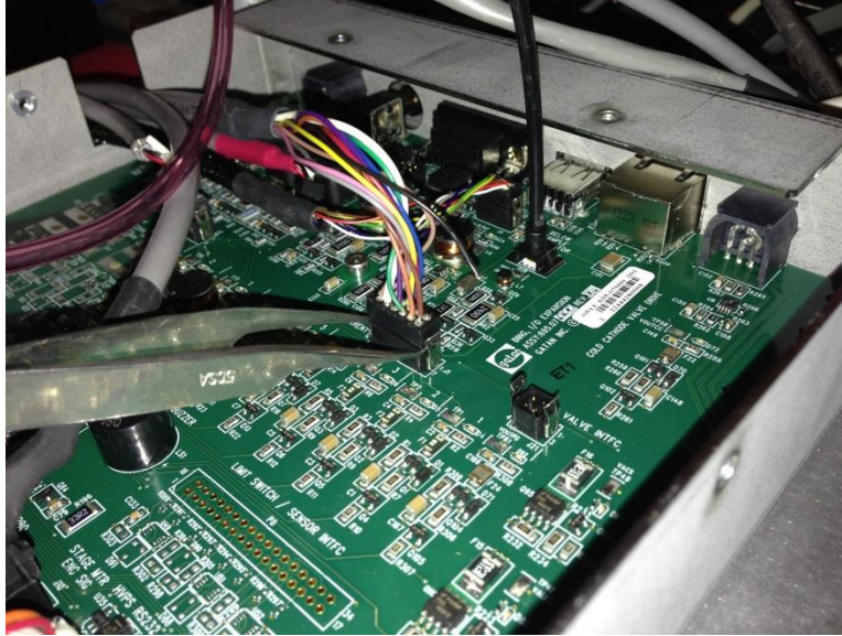
Figure 5-31 Removing cables from the I/O PCA.
