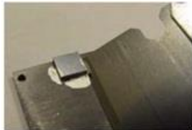
Figure 4-15 Removing the specimen from the sample blade
