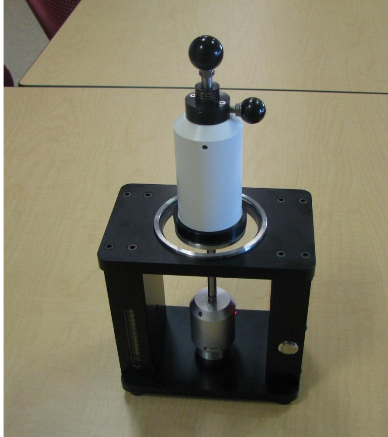
Figure 3-51. Transfer device grasping sample mount
