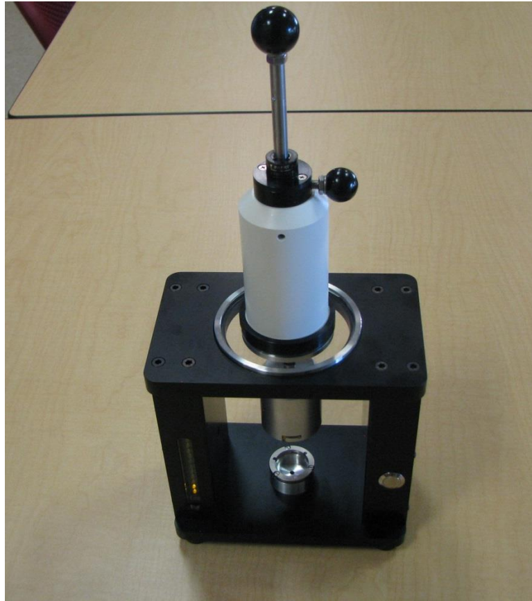
Figure 3-52. Transfer device lifting sample mount
