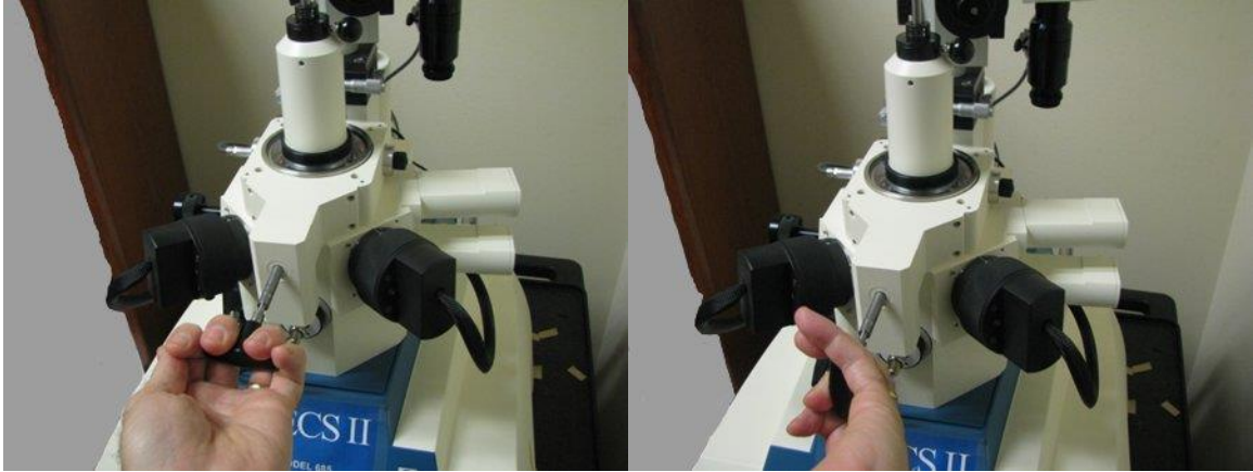
Figure 3-55. Opening the gate valve
