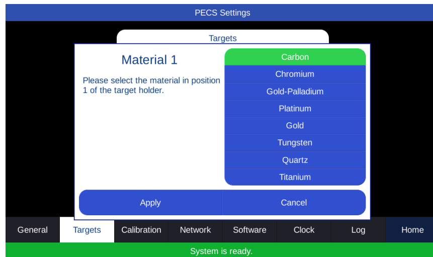
Figure 2-7. Target material selection
