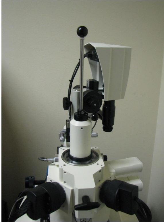
Figure 3-54. Transfer device on load lock
