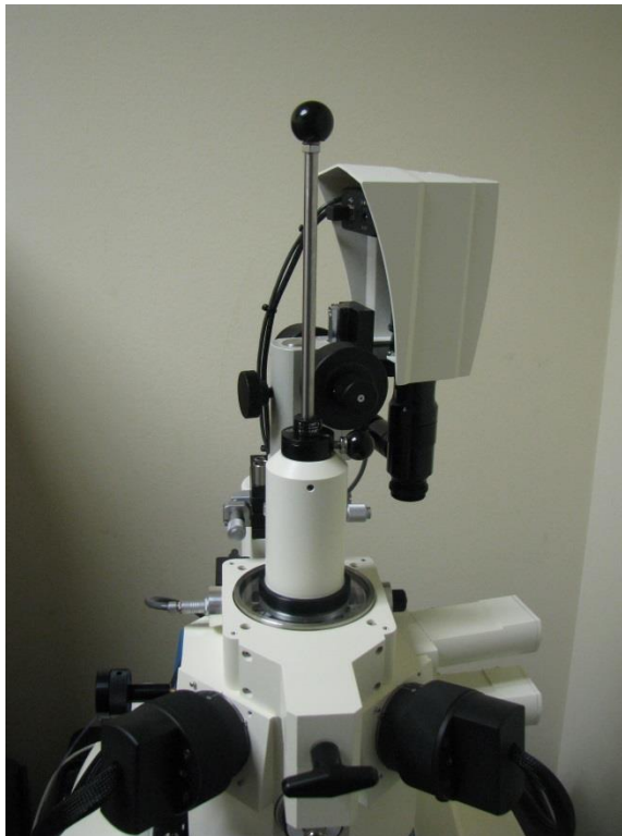
Figure 3-58. Transfer device on load lock
