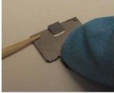
Figure 4-14 Scoring the Ag paint for specimen removal
