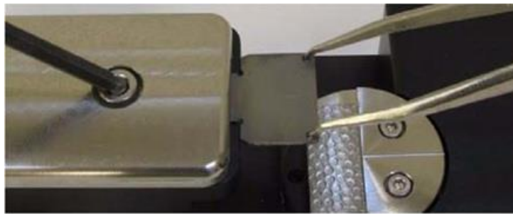
Figure 4-40 Verify the sample blade shoulders are fixed into position
