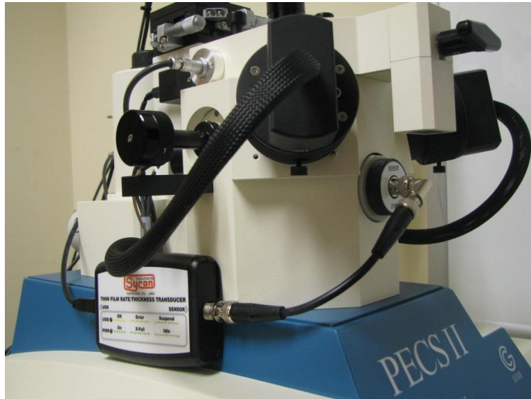
Figure 2-3. Film thickness monitor connections
