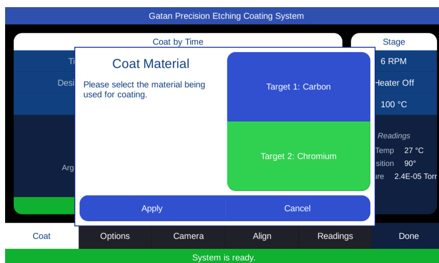
Figure 3-19. Setting the coating target.
