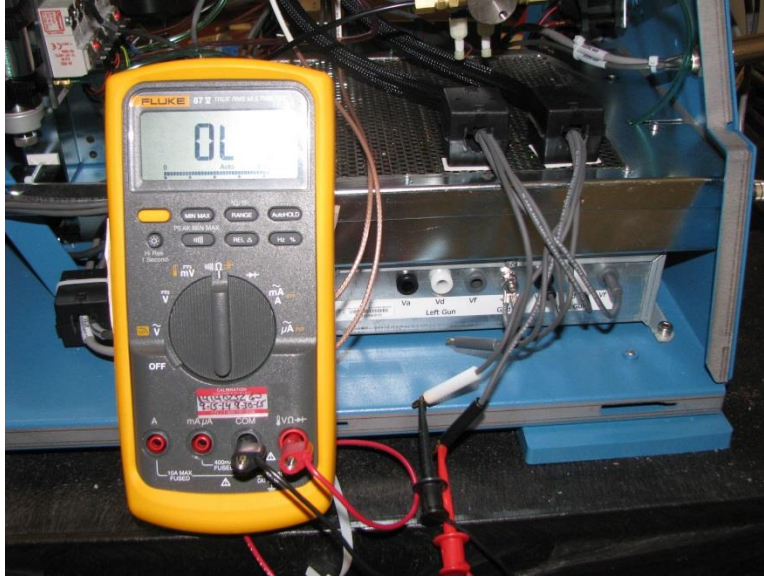
Figure 6-7. Resistance measurement showing open (good)
