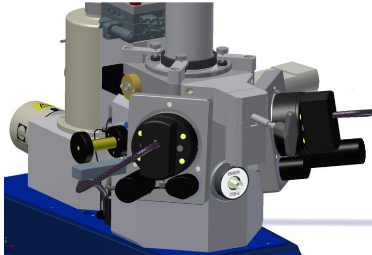
Figure 8-24. Gate valve open and latched
