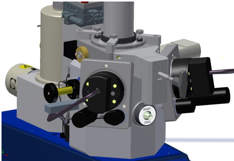
Figure 8-20. Tee handle out fully and rotated counter-clockwise
