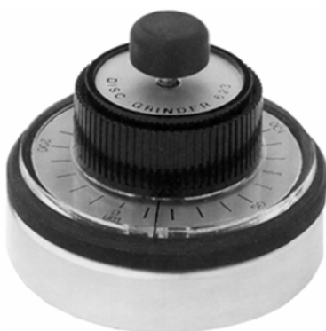
Figure 4-3 Gatan model 623 disk grinder.
