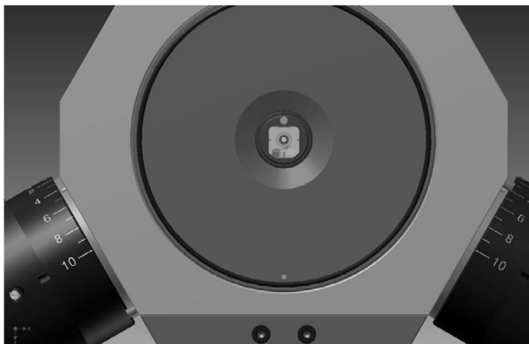
Figure 3-42 Specimen mount raised and in the Home position.
