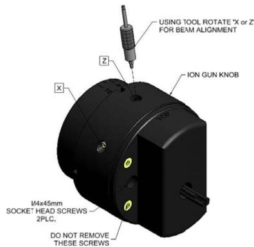
Figure 3-48 X and Z-alignment device screws.
