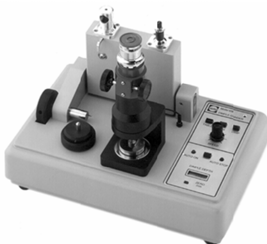
Figure 4-6 Gatan model 656 dimple grinder.
