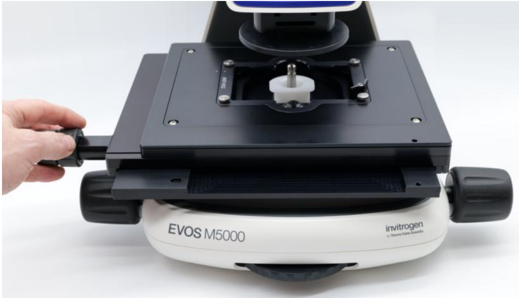
Figure 2 After removing the stage lock pin and moving the stage to access the shipping restraint.
