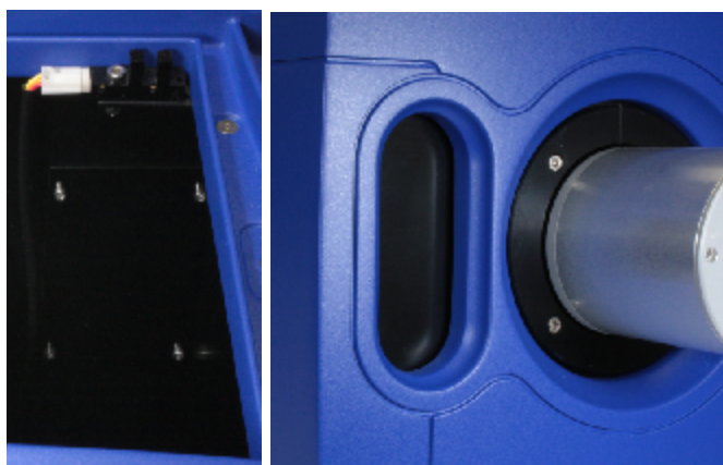
Figure 15: Location of the standard sample chamber bulkhead plate as seen from the inside (left) and from the outside (right) of the sample chamber
