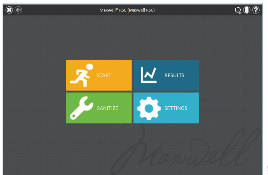
Figure 52. Maxwell® RSC ‘Home’ screen. When the Quantus™ Fluorometer is correctly connected to the Maxwell® RSC instrument, the “Q” logo is displayed in the upper right corner of the title bar.
