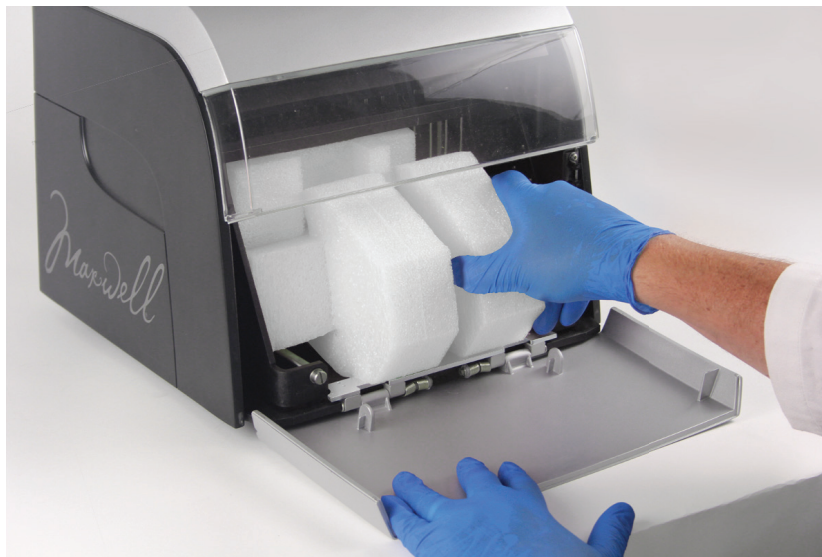
Figure 68. Placement of die cut foam in the Maxwell® RSC.
