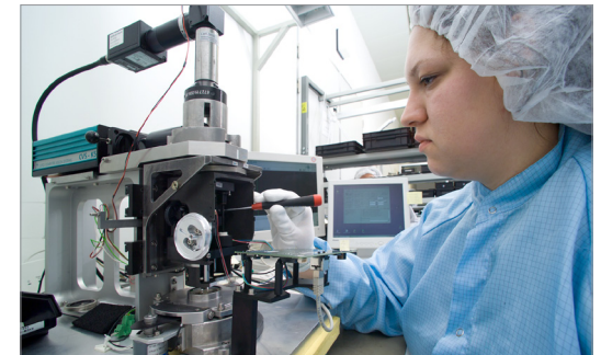
The zoom body adjustment device calculates the zoom control curve from around 7,000 reference points.
