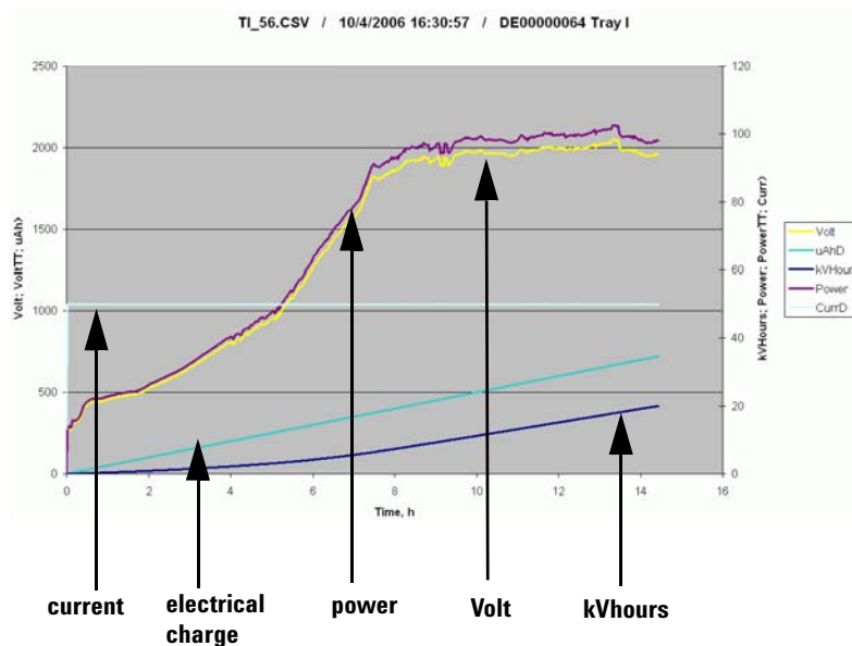
Figure 45 Example 1- typical results for the Protein test sample using the 3100 OFFGEL Low Res Kit, pH 3-10.
