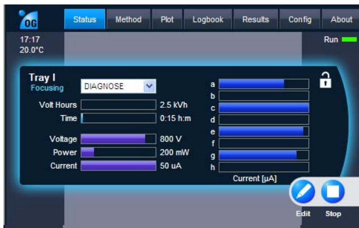
Figure 43 Typical current pattern on tray I when every second lane is filled with water.
