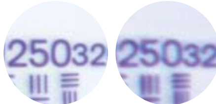
SMZ1000 Conventional model Comparison of resolving power and chromatic aberration factors
