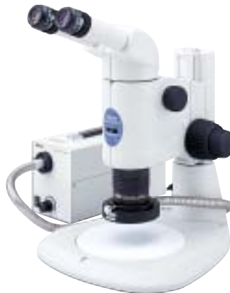
SMZ1500 configured with C-FIR Fiber-optics Ring Illuminator
