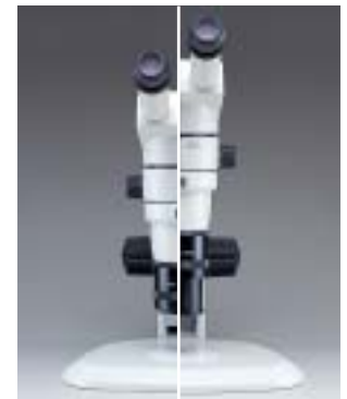
Ergonomic objective can be extended or retracted to adjust eye level.
