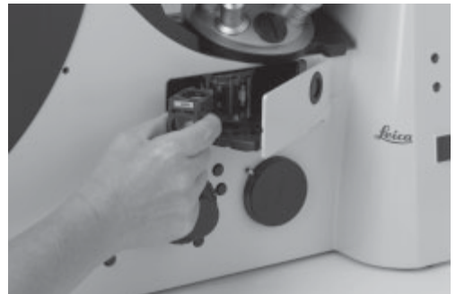
Fig. 68 Inserting or removing a filter cube
