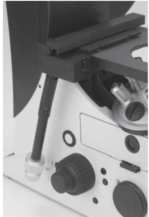
Fig. 25 Installation of attachable mechanical stage
