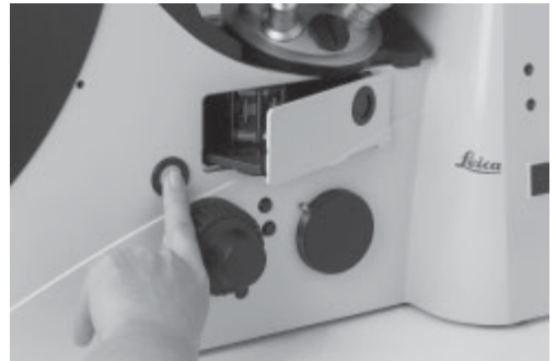
Fig. 68 Inserting or removing a filter cube
