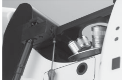
Fig. 24 Installation of attachable mechanical stage
