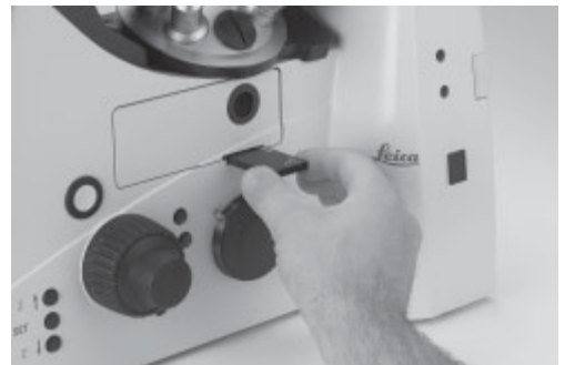
Fig. 110 Inserting the analyzer
