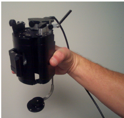
Figure 28. Proper Hand Position to Zero Diameter Arm
