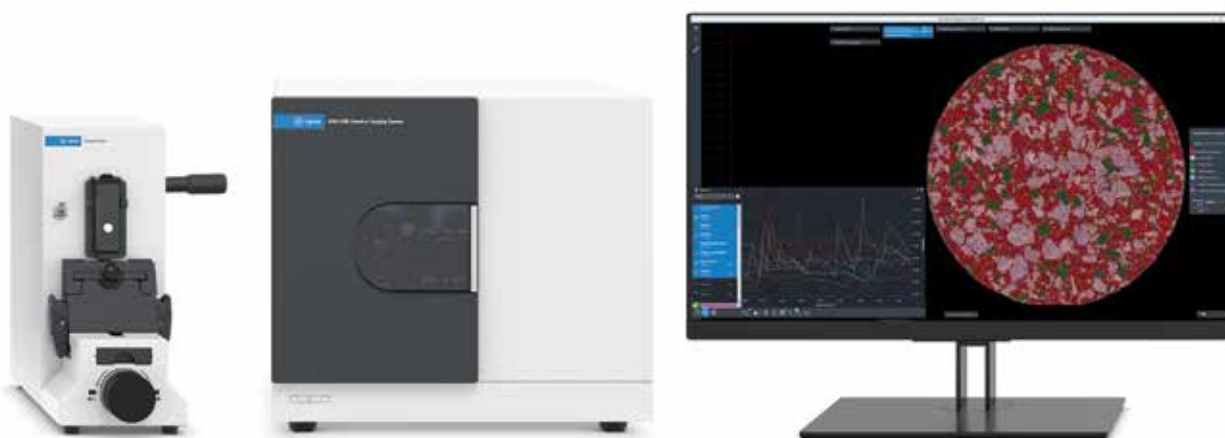
(From Left to right) Agilent Sample Planer, Agilent 8700 LDIR chemical imaging system and Agilent Clarity software analysis window
