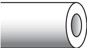
Figure 6 Properly cut tubing
