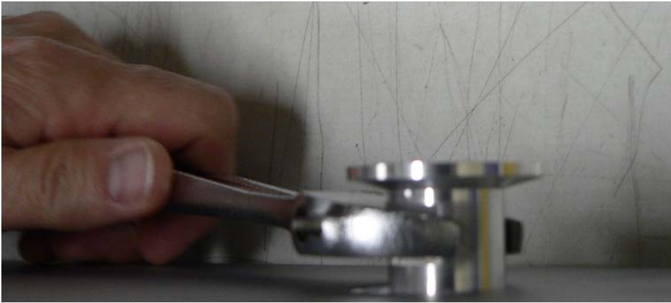
Figure B-7 Test Port Connection
