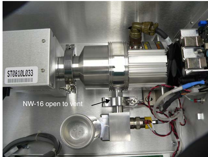
Figure B-76 NW-16 Vent
