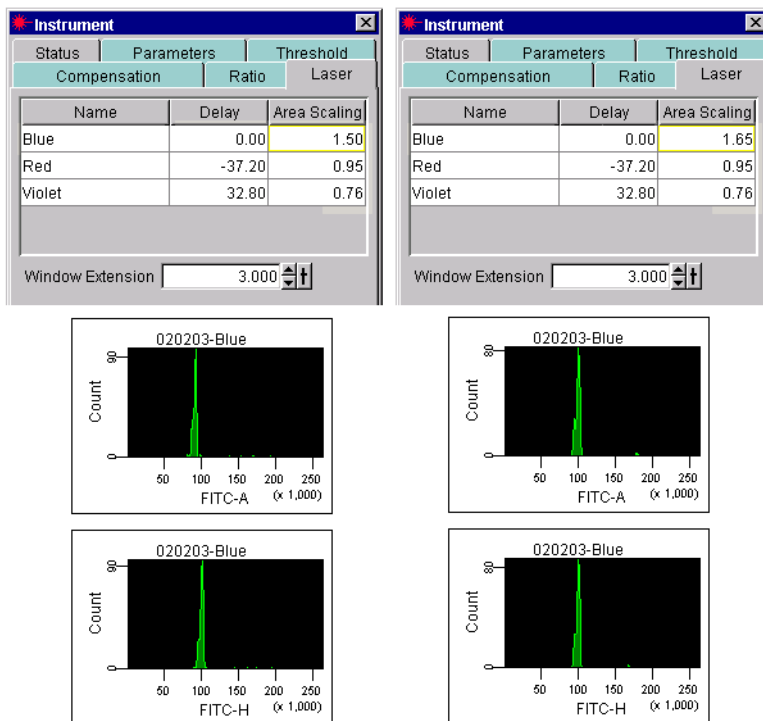
Figure 4-3 Blue laser area scaling before (left) and after (right) adjustment
