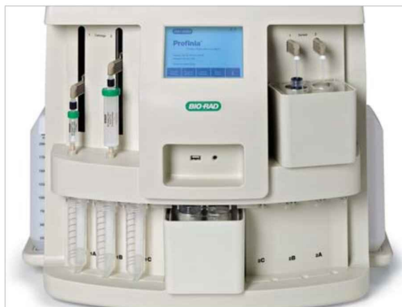
Cooling accessories are shown in place for the sample and fraction collection tubes.
