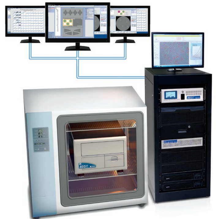
Figure 4. The IncuCyte ZOOM® system control and data access are enabled from any computer on your local network.
