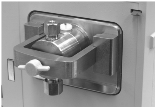
Figure 25 Pump Head Installed on the ProStar 210
