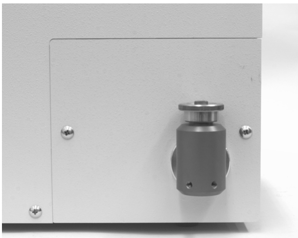
Figure 5 Internal Mixer in Place
