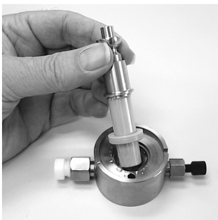
Figure 33 Piston Seal Removal
