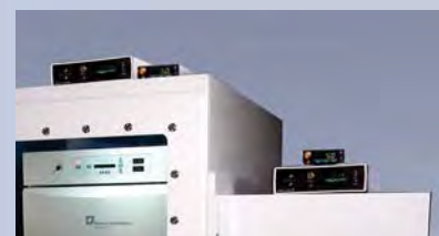
For extreme economy and flexibility, X3 processing chambers and buffer chambers can be controlled with modular independent controls such as ProOx and ProCO 2 .
