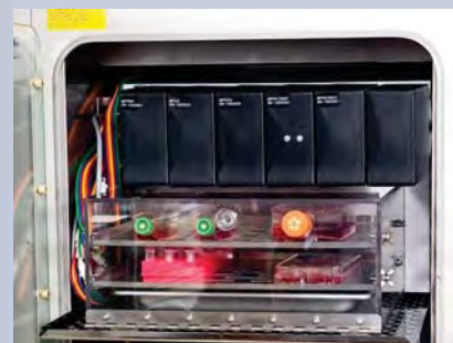
Multipod design dramatically reduces downtime for routine maintenance.
