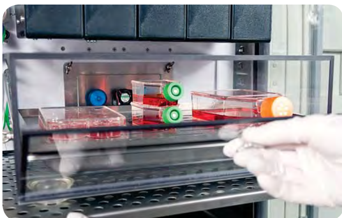
The adapter plate separates cells from sensors in pods with antimicrobial barriers.
