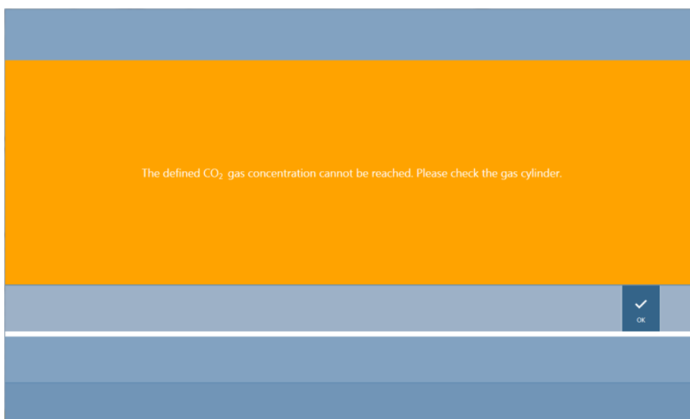
Figure 59: Stopping the gas alarm
