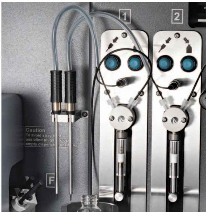
Figure 1 Reagent dispensers allow for easy and accurate reagent addition.
