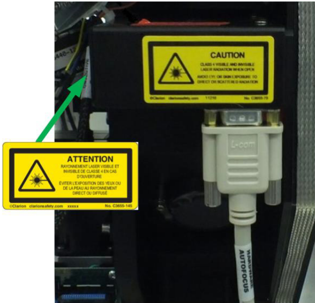
Class 4 Laser Non-Interlocked Caution labels - Hardware Autofocus Module
