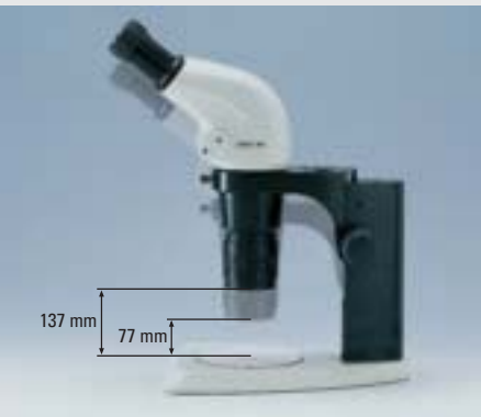
ErgoObjective 0.6× to 0.75×, working distance variable from 77 mm to 137 mm
