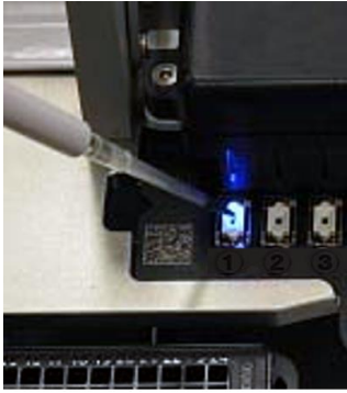
Blue LED illuminates the dispensehead on the cassette
