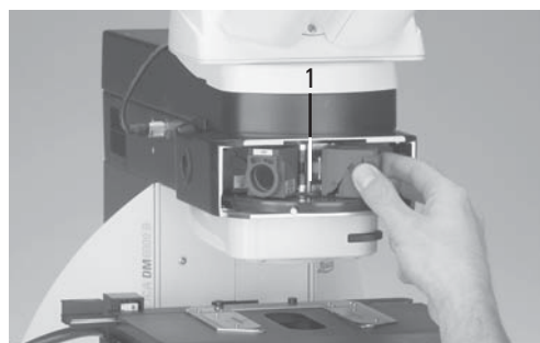
Fig. 31 Inserting the filter or reflector cubes 1 Mounting
