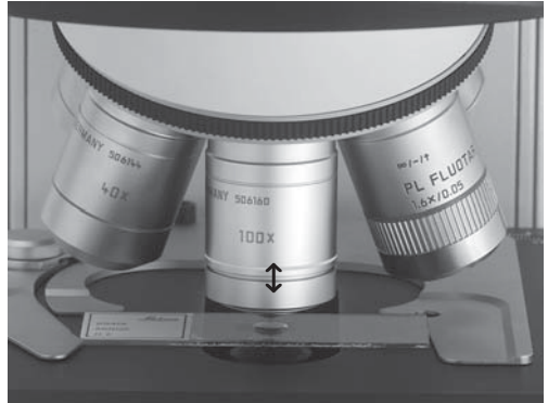
Fig. 71 Immersion objective (locked)
