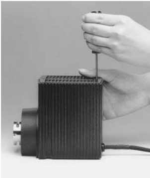
Fig. 15 Lamp housing 107/2 Releasing the fastening screw
