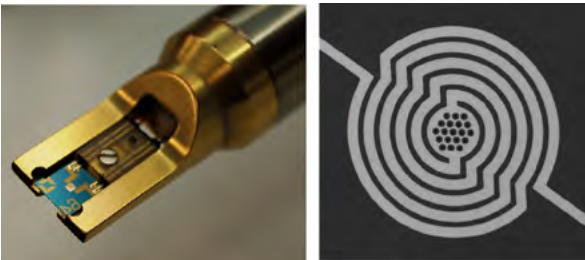
In-situ holder for heating experiments. The gas is introduced into the microscope through a separate nozzle.
