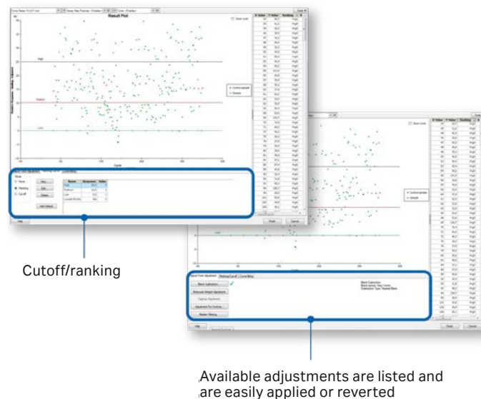
Fig 5. Using Result Plot , up to 5000 samples from several runs can be co-evaluated enabling easy selection of the samples of interest.
