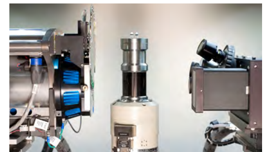
X-ray source (left), sample stage with tension/compression stage (center), and detector (right). Even with source to sample distances of several centimeters to accommodate in situ sample holders, voxel sizes below one micron can be achieved.
