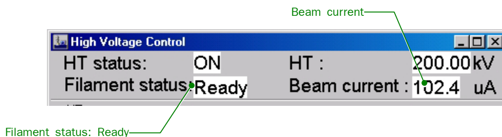
Fig. 5.12 High Voltage Control window
