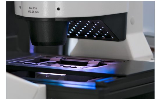
AI Sample Finder automatically detects your sample carrier, adjusts the focus, and finds your sample regions on the coverslip. Even with low-contrast samples, you will access relevant regions with just a click and start your experiment right away.
