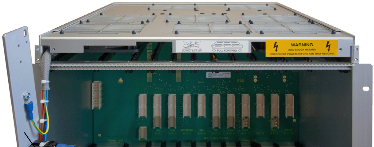
Front Panel with mains circuit breaker and cable
