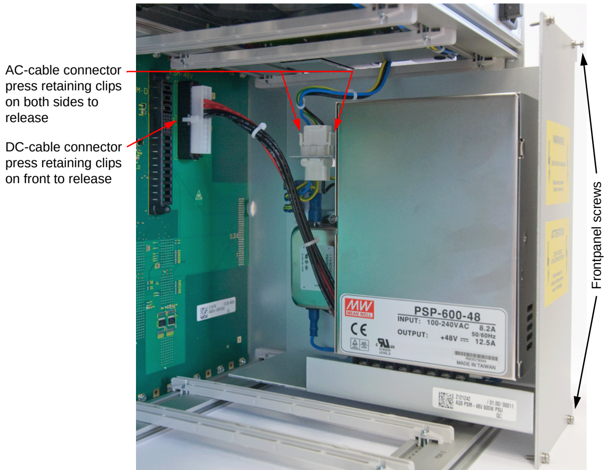
Figure 7.11 PSM-48V removal from mainframe
