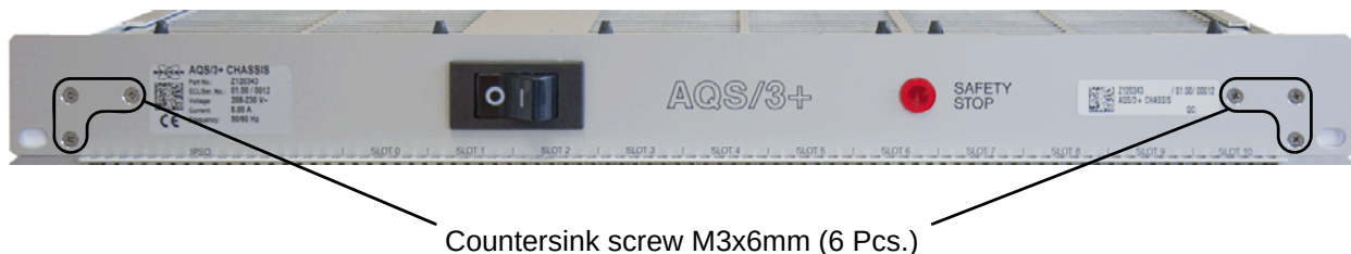
Figure 20.2 Fan Tray screws front side
