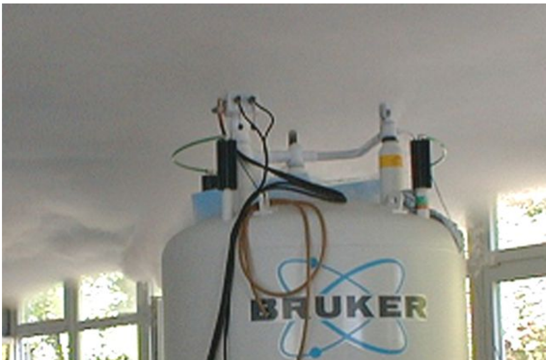
Figure 6.1: Magnet system during a quench
