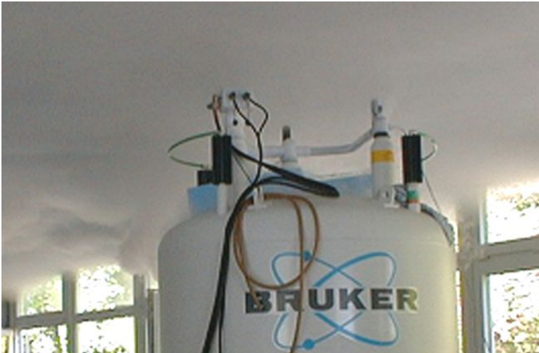
Figure 6.1: Magnet system during a quench
