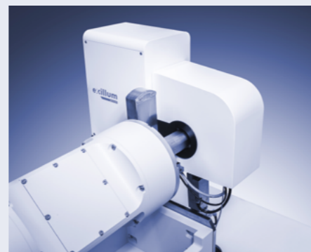
MetalJet source option: The highest X-ray flux available in the lab
