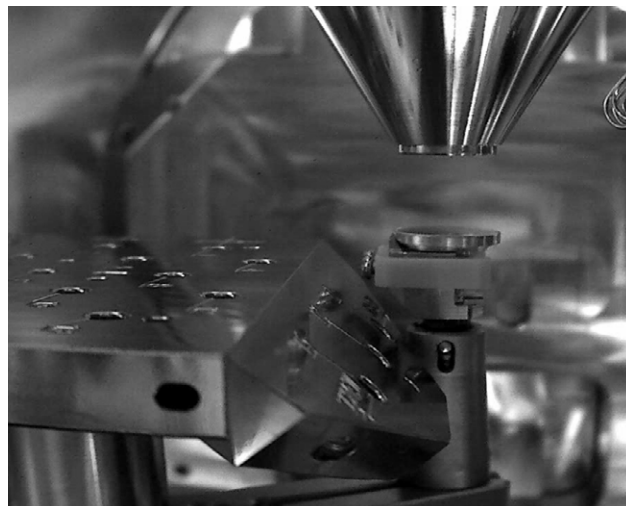
The pressure limiting aperture (PLA) is pre-mounted on the side of the multipurpose sample holder.
