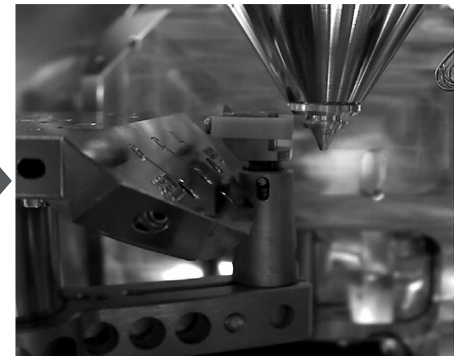
As soon as the PLA is mounted, the stage moves aside and the system is ready for low vacuum imaging up to 500 Pa chamber pressure.
