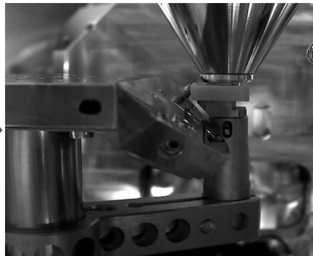
An automated routine moves the stage in order to insert the PLA when switching between high vacuum and low vacuum.
