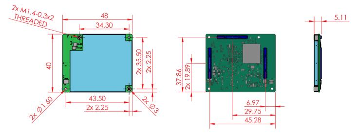
Figure 3. SoM dimensions (in millimeters)
