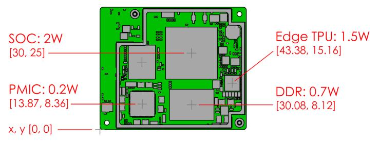
**Figure 4.** Power draw and ordinate locations (in millimeters) of top power components on the SoM while running the high performance test
