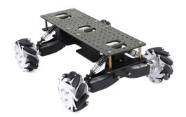
Mecanum Wheel Chassis with Suspension it is a 4-wheel drive mobile platform based on the Mecanum wheel. Each kit contains two left Mecanum wheels and two right Mecanum wheels. The four Mecanum wheels are connected to an independently controlled motor. Depending on the direction and speed of each individual wheel, the mobile platform can be forward, backward, lateral and any other desired direction or rotation.
